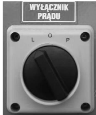
Figure 6 – The switcher set on unscrewing
