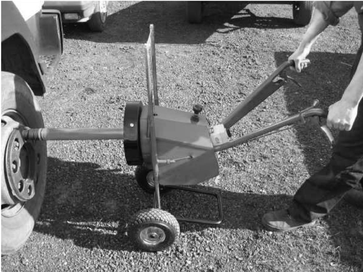
Figure 5 – Electric wrench driving method
