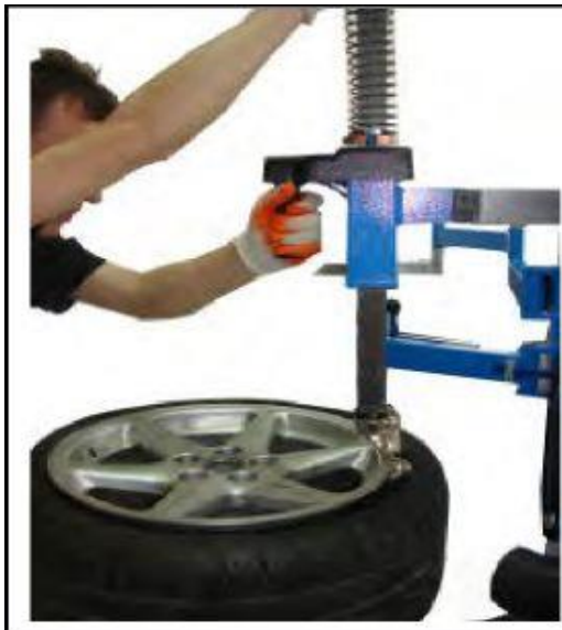
Fig. 8. Setting working head.
