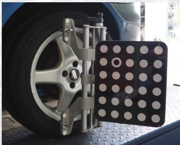
**Passive targets** attached to aluminum wheel clamps. The system quickly calculates the camber angle. No battery charging, no tangled power cables.
