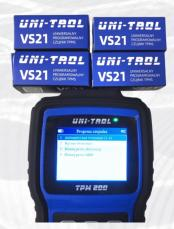
Programming of universal Uni-Trol VS21 sensors allows the use of one sensor in any car and optimizes the workshop's inventory.
