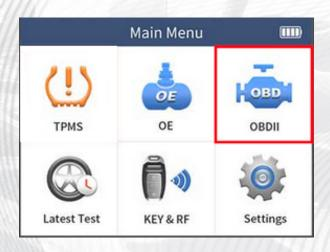
EOBD procedure allows you to diagnose EOBD protocol and check errors in the engine controller.
