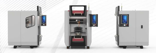
The movable control panel is always in the right place when working with the machine and after its completion returns to a special recess where it does not protrude beyond the machine. Under the touch screen there are control buttons and a special knob enabling the operator to very precisely control. The heart of the control panel is a computer running on Windows OS. It has a built-in WI-FI card that allows an operator to print a report or send it directly to an e-mail.
